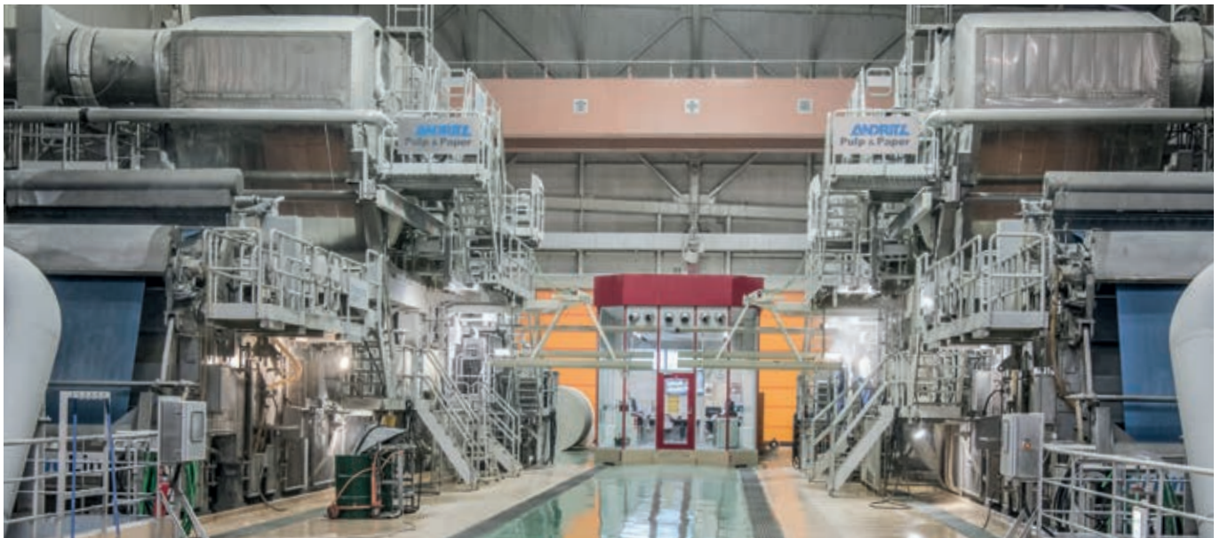
▲ The two identical PrimeLineCOMPACT machines are designed for a speed of 1,800 m/min and for a paper width of 2.8 m.
