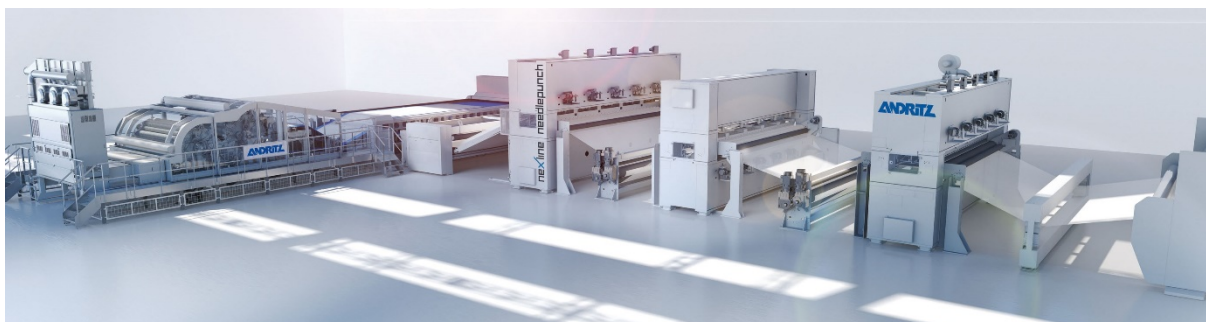
ANDRITZ high-capacity neXline needlepunch eXcelle line for production of geotextiles.
