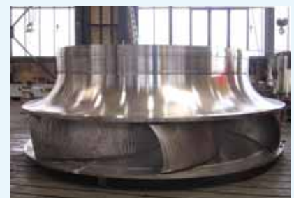
▲ Baixo Sabor pump turbine runner during fabrication in the workshop
