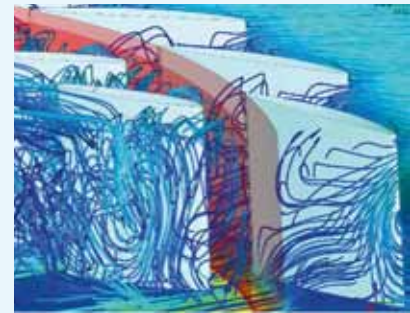
▲ CFD-calculated flow around the ring gate of Baixo Sabor Montante at 50%, 20%, 5% and 1% opening
