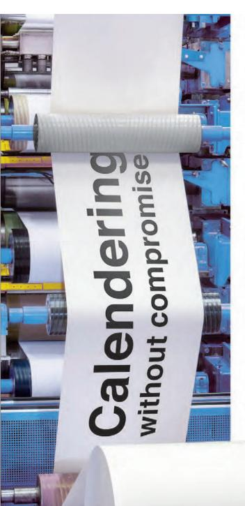
Bulk is an essential characteristic for some paper and board products. But one of the challenges of papermaking has been that achieving a smooth surface on paper has meant a considerable reduction in bulk. The latest innovation from ANDRITZ Küsters, the PrimeCal Y, overcomes the challenge by enhancing gloss and smoothness without compromising too much of the sheet's bulk and stiffness. The first unit has been sold and will soon ship.
