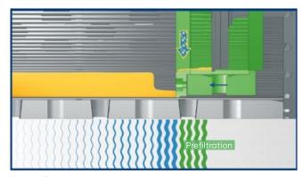
The prefiltration stage compresses and moves the cake into the main filtration zone. The liquid now drains off partly through the prefiltration and partly through the main filtration zone.
