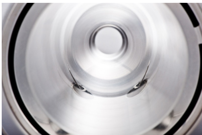
Detail of a washwater hydrocyclone for mercury reduction (patented by ANDRITZ).
