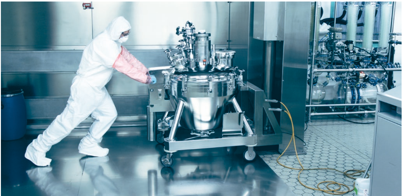
Filling, transport and product discharge with one single mobile dryer.
