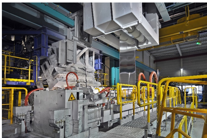
ANDRITZ hot-dip galvanizing section.
