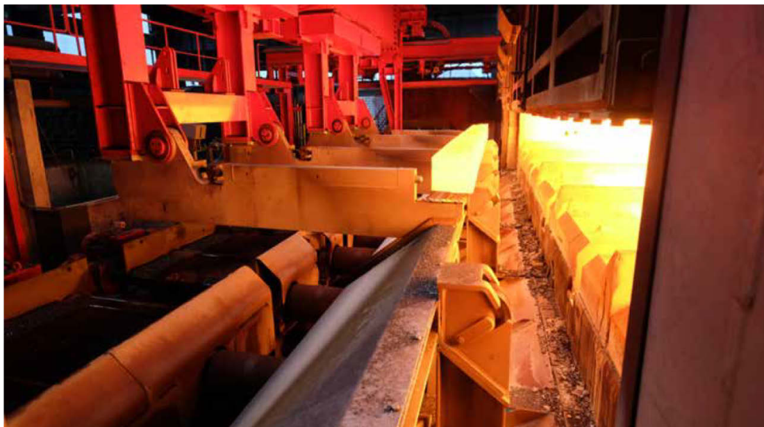
Removal of billets with manipulator.
