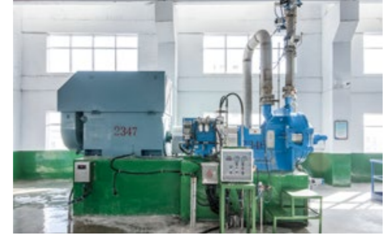
The P-RC APMP system using the very latest TwinFlo TF refiner from ANDRITZ
