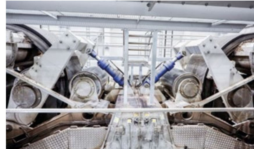
Two new-generation HQ-Press bark presses at wood processing increase energy value of bark.
