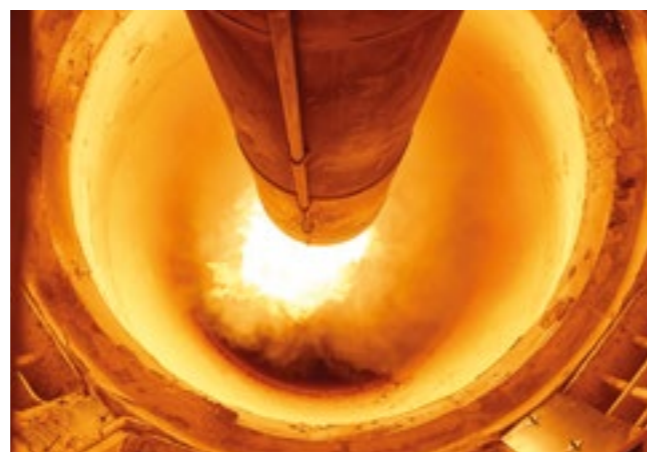
View from the inside of the lime kiln, using wood powder
