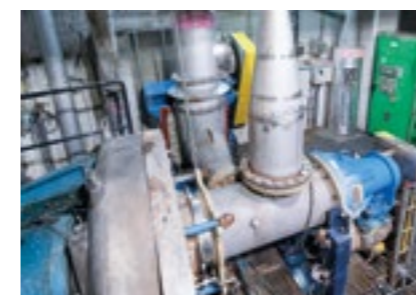
The BR1 reject refiner needed a complete tailor-made solution to ease plugging
