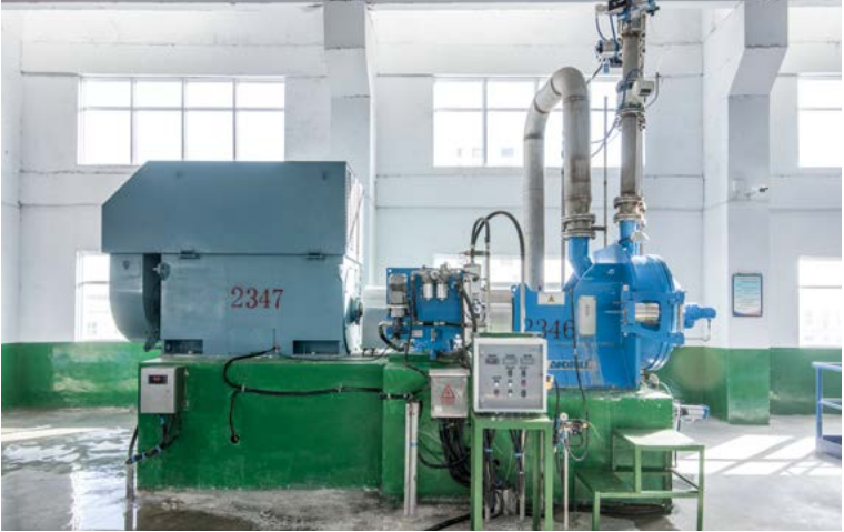
The P-RC APMP system using the very latest TwinFlo TF refiner from ANDRITZ
