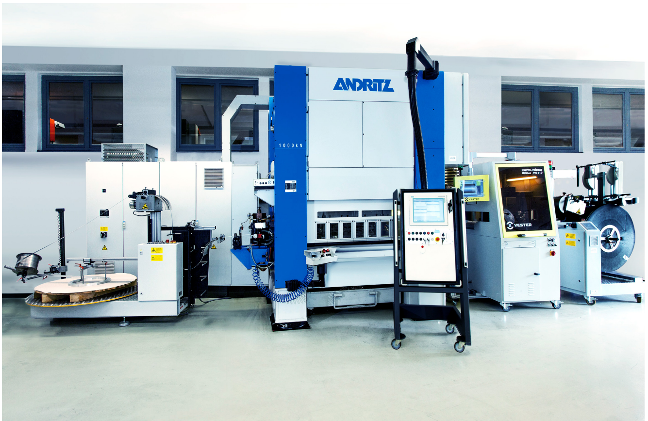
Conventional ANDRITZ automatic stamping press with coil handling line and quality control system for stamped parts.
