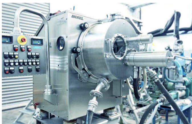
Krauss-Maffei peeler centrifuge equipped with the recently launched pneumatic discharge system.
