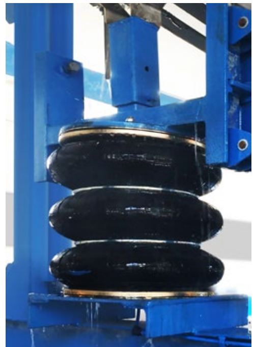
Bellows for vacuum box lifting device
