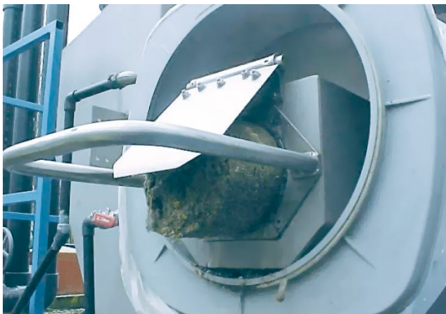
An efficient screw compactor for easy transport of waste
