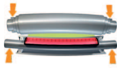
Increased line force at the edges
