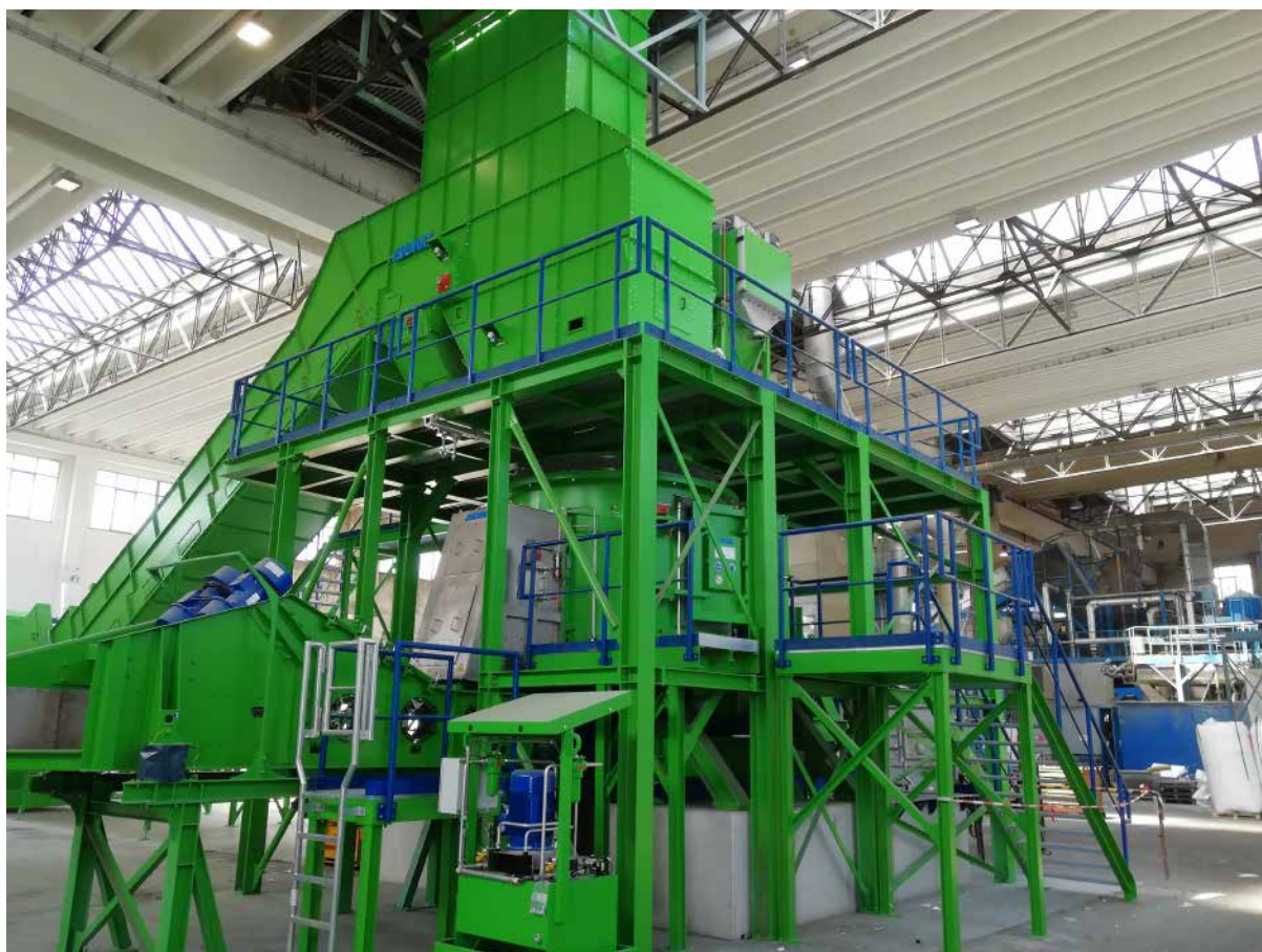
Refrigerator recycling plant including the ANDRITZ Universal Cross-Flow Shredder QZ 2500.
