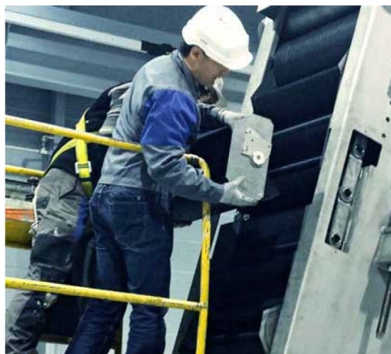
Aqua-Screen P and T: Filter elements can be dismantled from the front in less than 30 minutes.
