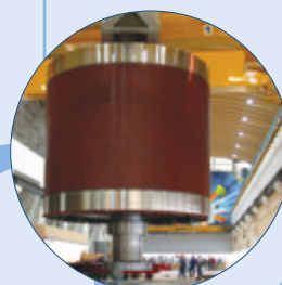
Goldisthal Germany, the first asynchronous variable speed pumped storage unit (330 MVA) outside Japan in 1997
