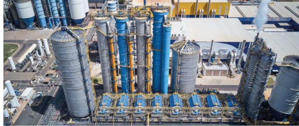
The new hardwood fiberline ensures low operating costs, low emissions, extremely high washing efficiency, and excellent fiber quality. The capacity (6,120 adt/d) is the highest in the world for a single fiberline.
