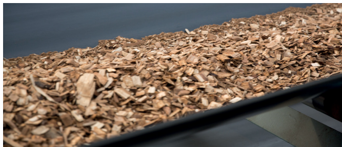
▲ ANDRITZ provided the basic engineering and chip screening technology ensuring that incoming chips are of optimum size for the cooking plant. Oversized chips are treated in a new ANDRITZ rechipper.
