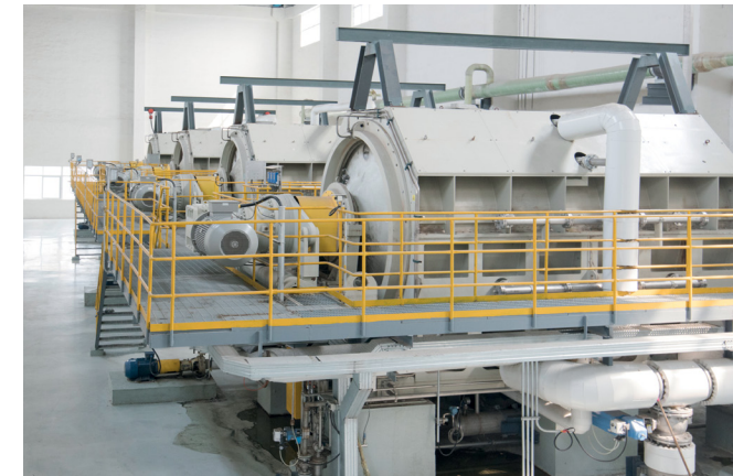
▲ Following the new continuous digester are multi-stage DD Washers for brownstock washing and post-oxygen washing, and a single-stage DD washer after every bleaching
