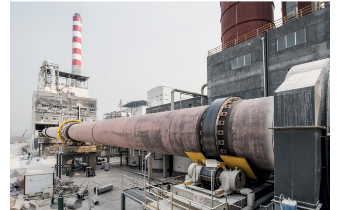
▲ The mill's new white liquor plant from ANDRITZ has capacity to produce 4,800 m³/d of white liquor. The LimeKiln shown here can produce 400 t/d of returned lime.
