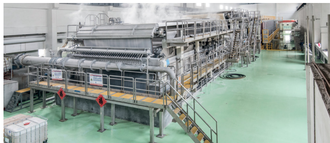
▲ ANDRITZ's delivery of the pulp drying plant (1,200 admt/d of kraft or 950 admt/d of dissolving pulp) has some advanced and innovative energy-saving technologies to reduce operating costs.
