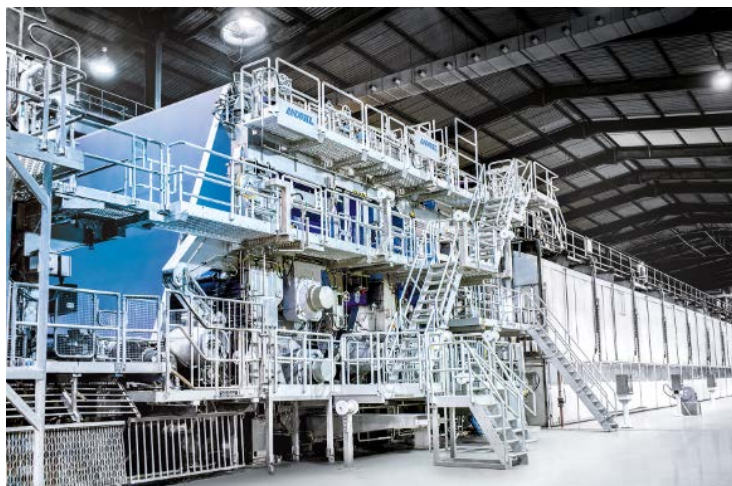
ANDRITZ PrimePress X shoe press for gentle dewatering and bulk savings.
