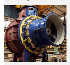
BEW owns five run-of-river power stations along the Iller River, among these are the Illerstufe V (Fluhmühle), the Illerstufe VI (Legau) and the Illerstufe VII (Maria Steinbach). All these hydropower stations were built between 1938 and 1944 and are equipped with Straflo turbines – single regulated axial turbines with a fixed runner position and integrated generator pole shoes located on the outer rim of the runner blades.
