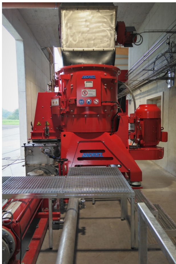
ANDRITZ Universal Cross-Flow Shredder Bio-QZ in the biogas plant of Holzhof cheese factory
