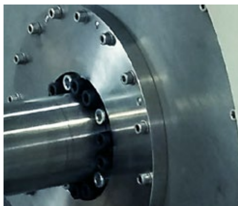
Internal clamping set to secure the drum body to the shaft, non-wetted section
