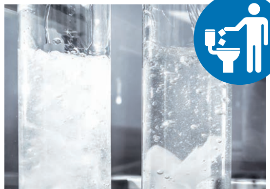
Dispersion of wipes produced by the Wetlace™ technology
