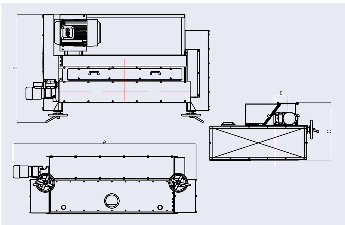
The crumbler type SCR enables by-pass, precisely adjustable rollers, integrated dual sampling spots and uniform feeding into spring loaded rollers.
