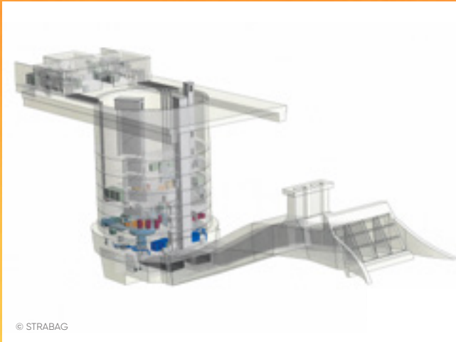
The final concept is based on a shaft type powerhouse, hosting two pump turbine motor-generator units with 125 MW each.
