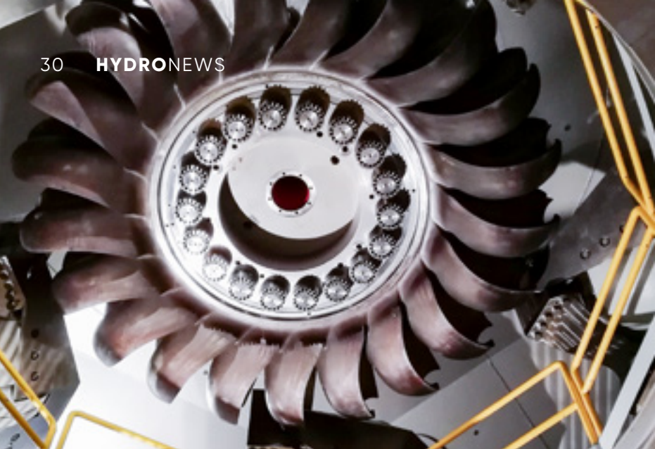
The new Pelton turbine completes the existing reversible pump turbines and features extremely good part load behavior.
