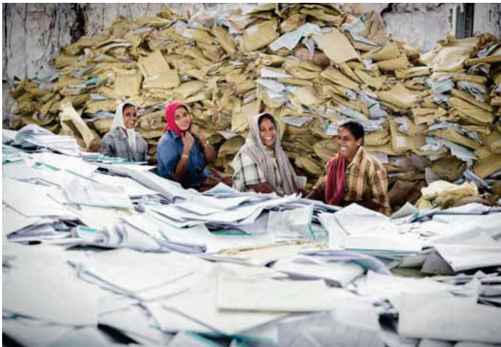
▲ The raw material mix consists of 80% sorted office paper and 20% old magazines. The ANDRITZ deinking and bleaching technology achieves a final brightness up to 87% ISO.
