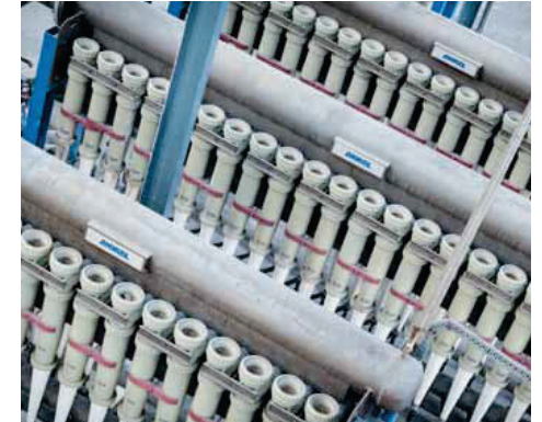
▲ After pulping, the next task is the removal of heavy particles in a two-stage cleaning system, preserving the life of downstream equipment.
