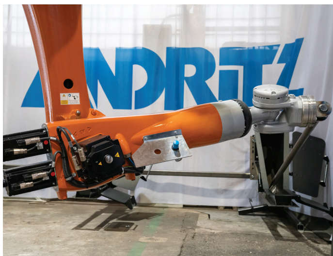
Smelt spout robot in showroom (left) and in operation at mill (right)
