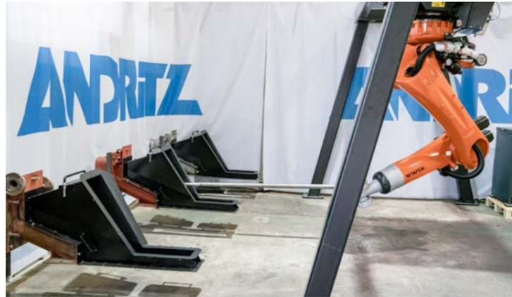
and one robot can clean up to three spouts using a long-reach arm. Despite its power, the robot recognizes the position of the spouts through positioning sensors and does not damage them during the cleaning procedure. On the end of the arm is a specially designed tool that cleans away the solidified smelt.
