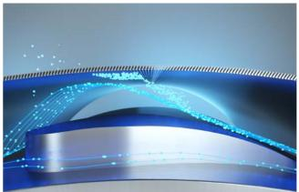
The smooth pressure zone provides effective flow distribution over the cylinder surface reducing energy consumption. Additionally, the strong suction zone reduces thickening and improves runnability.
