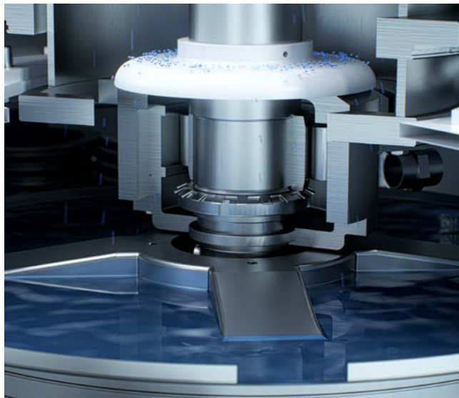
Splash guard to protect the pulley
