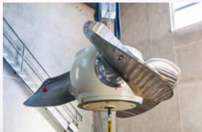
Picture 2: Fish-friendly runner enhancement for the Eddersheim hydropower plant in Germany.
