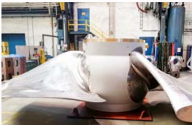
Picture 1: Turbine runner for Monsin hydropower plant in Belgium with strictly fish-friendly design
