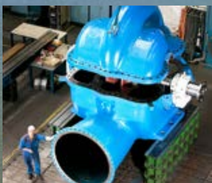
Hui Nan Zhuang, 8 horizontally split double-suction pumps
