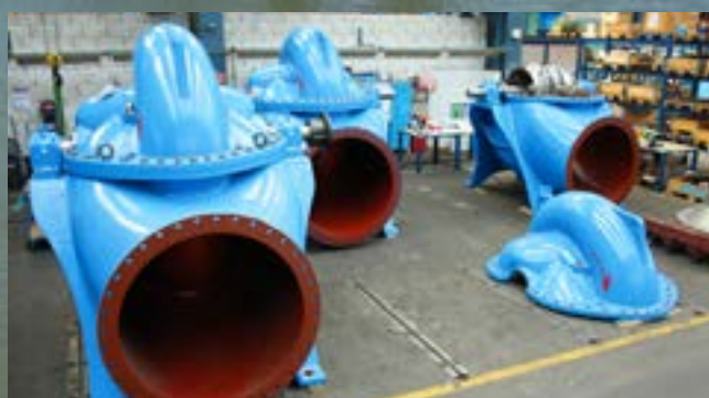
Xijiang Intake Pumping Station, 12 double-suction pumps
