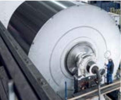
Tissue: Carta Fabril, Brazil. Workshop impression of the steel Yankee with a 22 ft. diameter.
