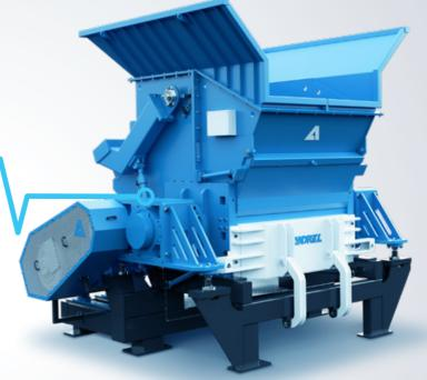
t was a first for ANDRITZ and its customer and a landmark in refuse-derived fuel production. The July 2019 installation of an FRX3000 at SRP Sekundärrohstoffe in Pöchlarn, Austria, is perhaps the first time a pre-shredder has been used to process high-caloric input material down to 35 mm particles for use in cement plants.
