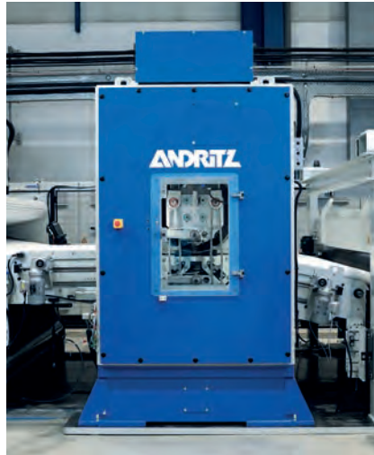
ANDRITZ neXloom pre-needler orbital type cylinder
