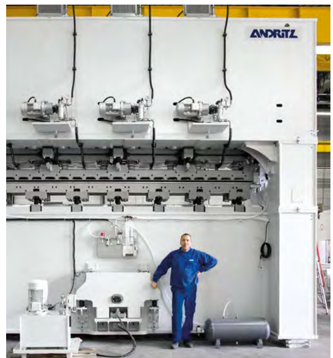
RIB structuring SDB-1 in 4.40 m working width
