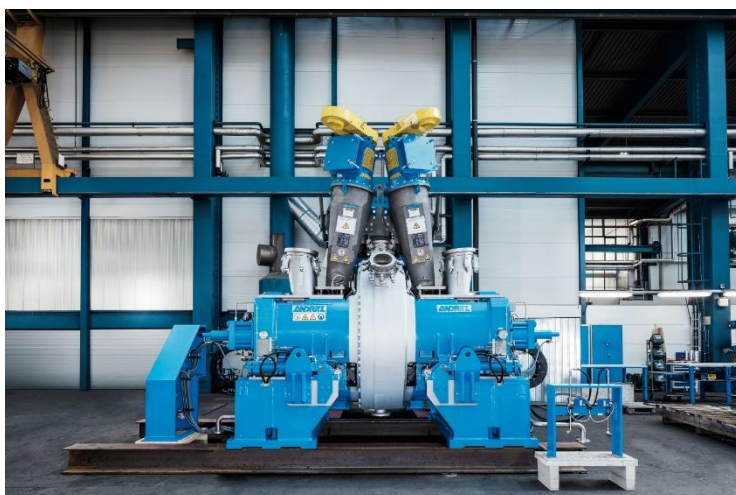
ANDRITZ TX68 refiner with newly developed feeding system
