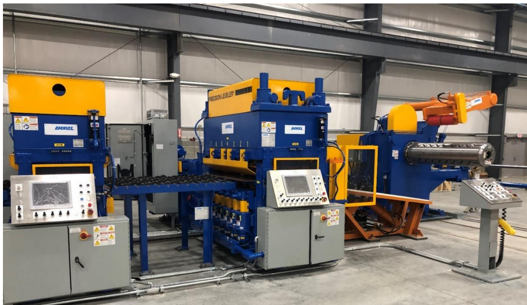
Entry End of the Cut-To-Length Line with Uncoiler, and two Precision Levelers
