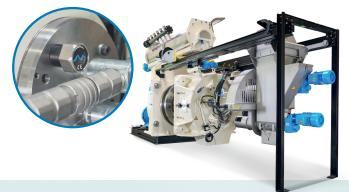
The Metris Vibe sensors developed by ANDRITZ form the basis of effective and low-cost condition monitoring. Small, wireless, and energy self-sufficient, our Metris Vibe sensors can be easily installed in large numbers at all the relevant points, providing a continuous data stream on vibrations and temperature.
