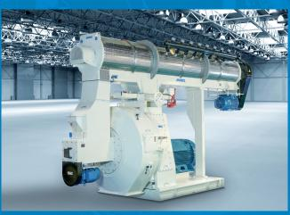
The constant monitoring of critical components enables effective and timely fault detection for rotating parts of extruders, expanders, pellet presses, and hammer mills, for both ANDRITZ AND non-ANDRITZ equipment. These machines have high precision and costly inner work. Based on alarms and recommendations, Metris Vibe enables proactive planning and actions for predictive maintenance of your plant, keeping it consistently healthy and high performing.
