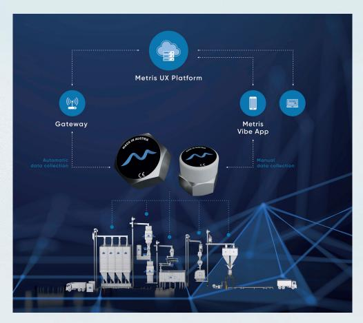
Metris Vibe sensors work wirelessly, communicating via their own secure system, without interfering with your IT systems.
