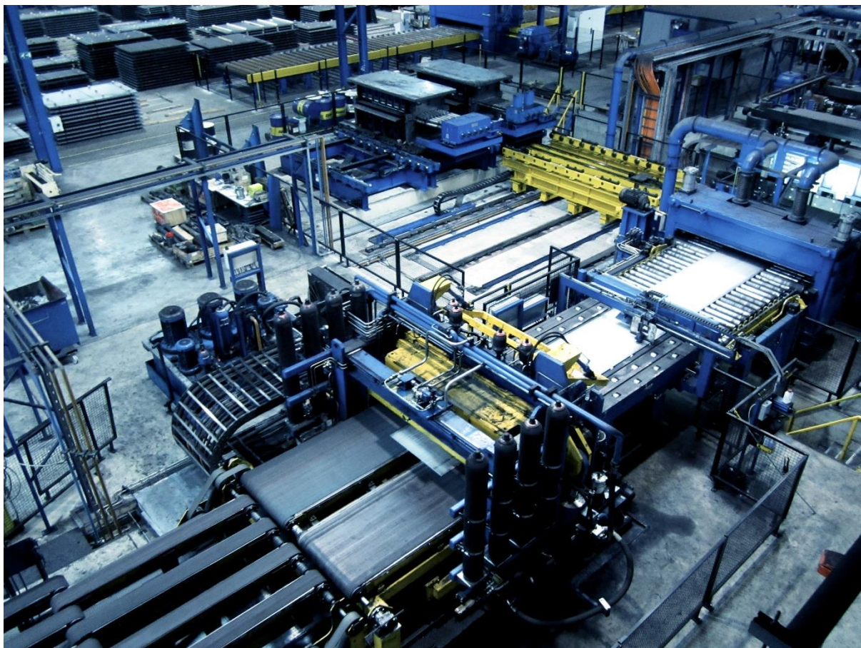
Cut-to-length line with heavy-duty leveler
