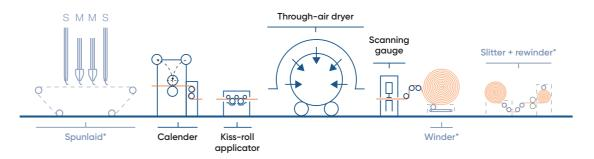
ANDRITZ spunlaid finishing line for hygiene and medical end-uses, 8-80 gsm
