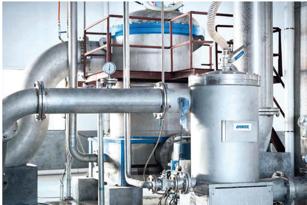
▲ A complete paper machine approach system from ANDRITZ is also in place. A ModuScreen headbox screen plays an important role in delivering stock to the new machine.
