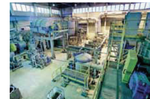
▲ ANDRITZ also delivered a new recycled fiber processing line and machine approach system with a capacity of 800 t/d to bring high-quality stock to PM7's new headbox.
