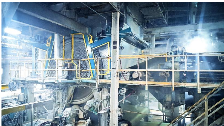
Close-up view of the PrimeDry Hood with Yankee at Cascades Tissue Group Wisconsin.
