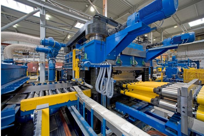
Heavy-plate leveler for ultra-high strength steel
