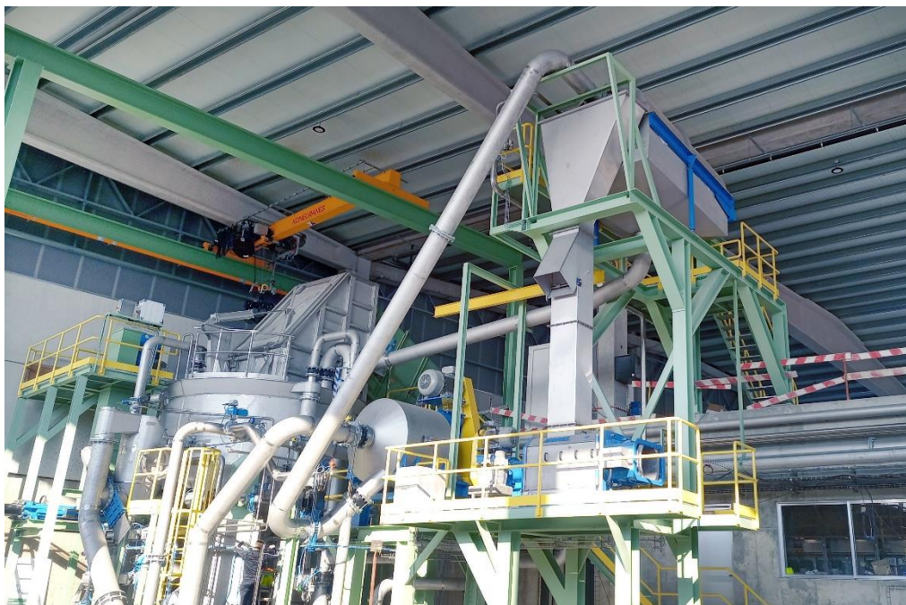
Complete LC pulping system supplied by ANDRITZ at Papeleira Coreboard
